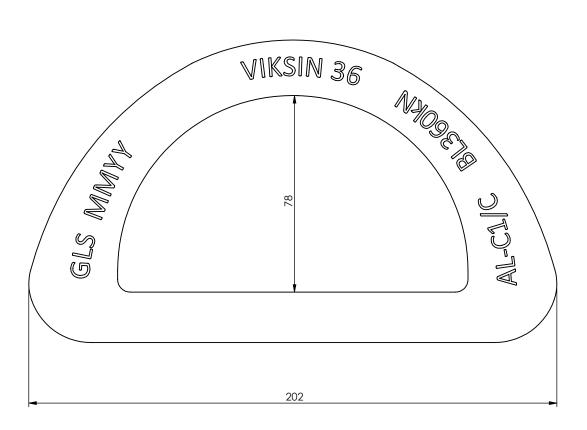
Marking 1: Batch number MM = Month YY = Year, Marking 2: VIKSIN 36 = Brand name indication, Marking 3 = Type indication 360kN = max load
