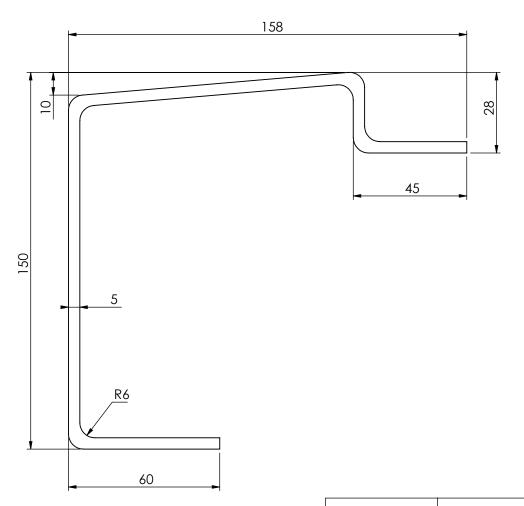
Article nr: Dimensions: 0101031580 4.5 x 158 x 150 x 3000mm (standard size) On request 4.5 x 158 x 150 x (L<3000mm)
