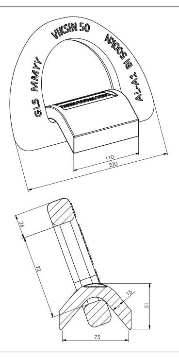
Marking 1: Batch number MM = month YY = Year, Marking 2: VIKSIN 50 = Brand name indication, Marking 3 = Type indication, 500kN = max load
