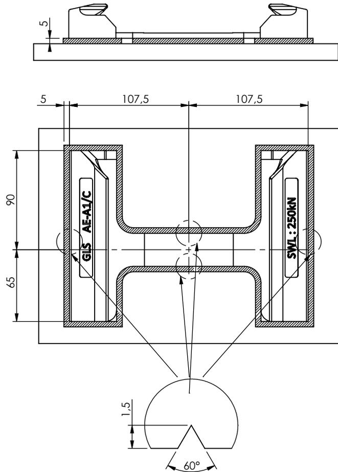
1. Welding preparation: Clean the locations for the weld on the foundation as well as on the connection area. Clean all the dirt, rust or any residual paint.
